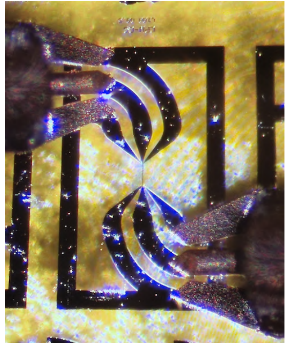
(b) Enlarged microscopic picture of the YIG sample and the specially shaped CPW transducers and the attached sensors of the picoprobes for the DE mode.
